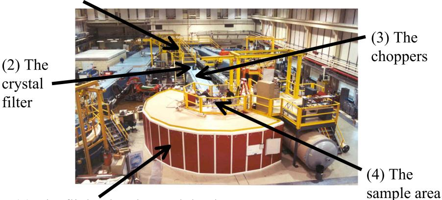
(5) The flight chamber and the detectors
